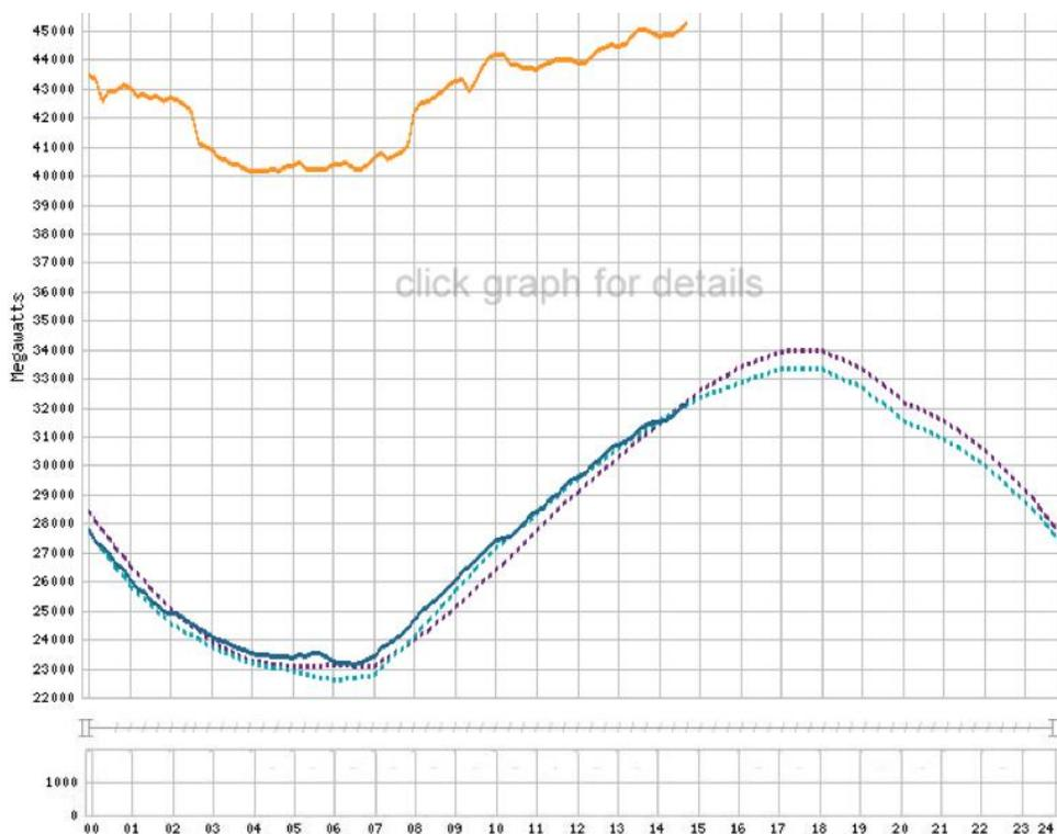
The vertical scale (too small to read I’m afraid) is the amount of power, measured in megawatts, while the horizontal scale is the time, starting at midnight. Dotted lines represent two forecasts: “day ahead” and “hour ahead”, while the solid blue line is the actual demand. This particular graph was made at 3 PM on July 4<sup>th</sup> (and the demand at that instant was still below the peak, which was
