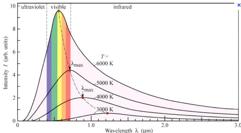
Figure 1: How the amount of radiation from surfaces of a fixed area is distributed over wavelengths depending upon the temperature of the surface.
